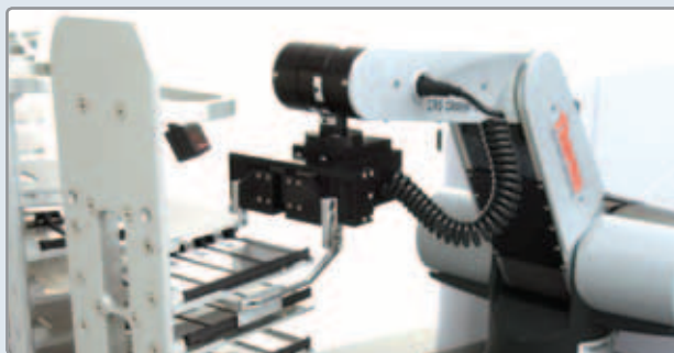
Clemex Maestroscope selects sample holder from hotel (glass slides or microplates)
