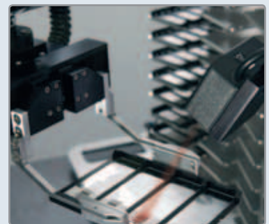
Bar codes are scanned for sample identification
