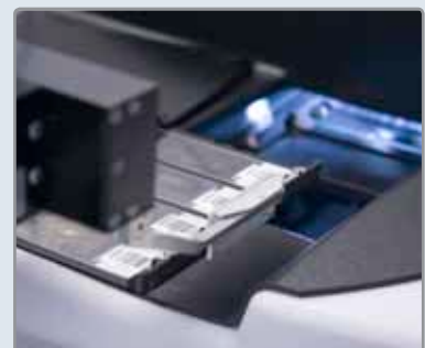
Clemex Maestroscope places the samples in analysis position
