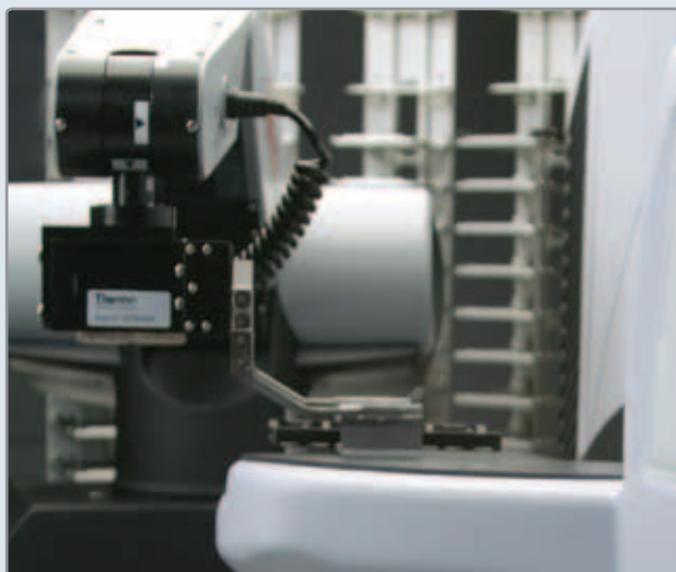
Clemex Maestroscope positions sample holder in stage plate
